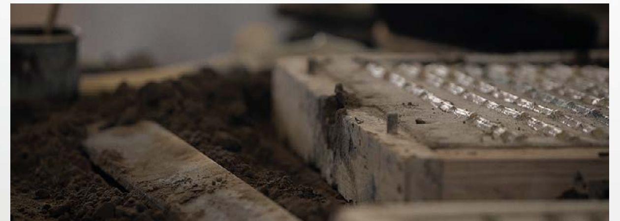
The brass casting process is made with sand, fire and brass. The melted brass fills the shapes and textures left on the sand by the branches and the leaves.
